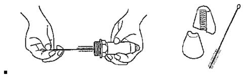
**IMPORTANT:** DISCONNECT THE TOOL FROM THE AIR SUPPLY OR SWITCH OFF AT VALVE (55). REMOVE NOSE ASSEMBLY OR SWIVEL HEAD COMPONENTS. All operations should be carried out on a clean bench, with clean hands in a clean area. Ensure that the new oil is perfectly clean and free from air bubbles. Care MUST be taken at all times, to ensure that no foreign matter enters the tool, or serious damage may result.
